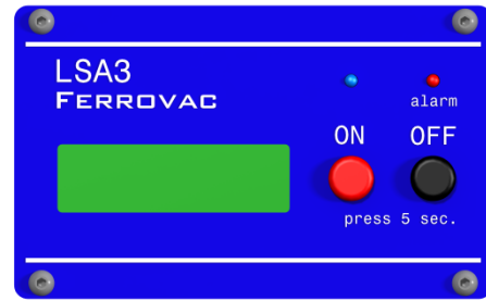
Figure 7: Front of the LSA controller.
