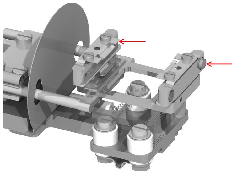
Only one of the two styles of sample carriers can be inserted at any given point.
